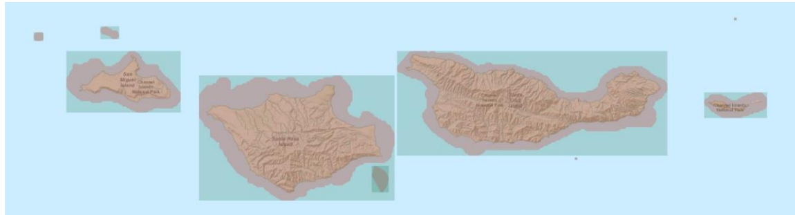
Unsafe areas, shown in red, surrounding the Channel Islands. The blue rectangles are bounding boxes used in a search algorithm.
