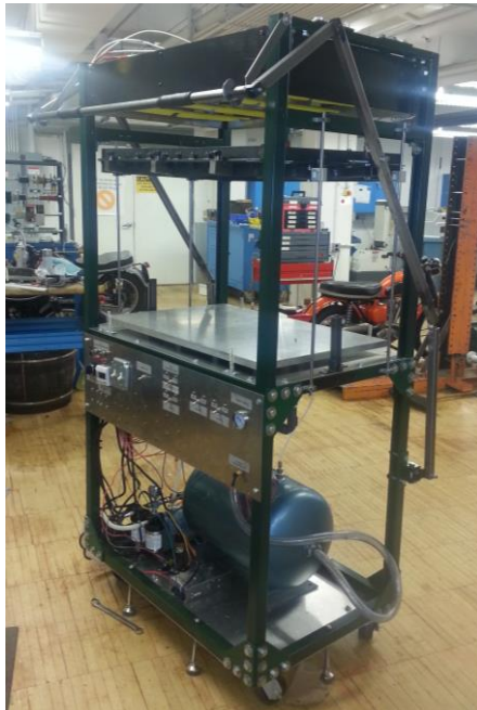
The final thermoforming machine with the mechanism raised
