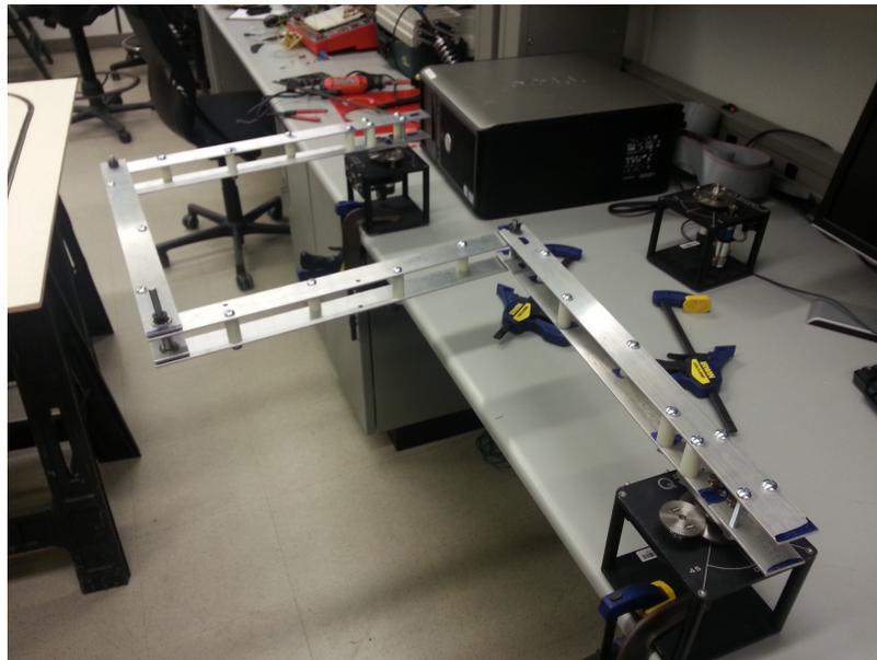
Figure 2.1: Quanser Five-Bar Linkage System
